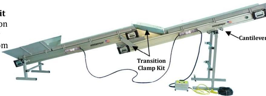
A cantilever set on a leg kit enables the discharge conveyor to overhang.
